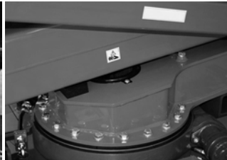
Fig. 96 Example potential shearing risk zone 2
