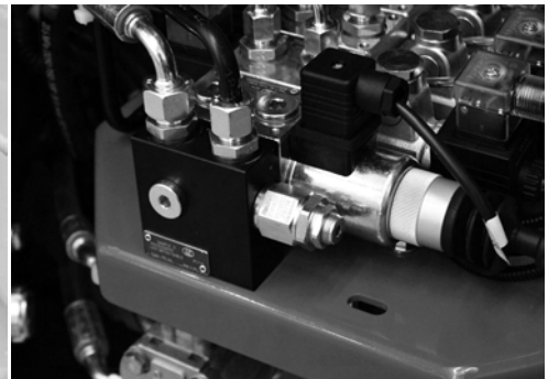
Fig. 9 Ground part pressure relief valve 1
