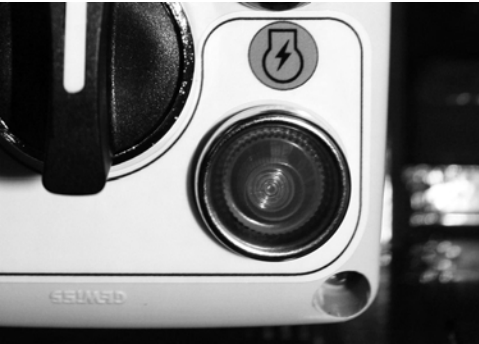
Fig. 111 Emergency control panel lamp
