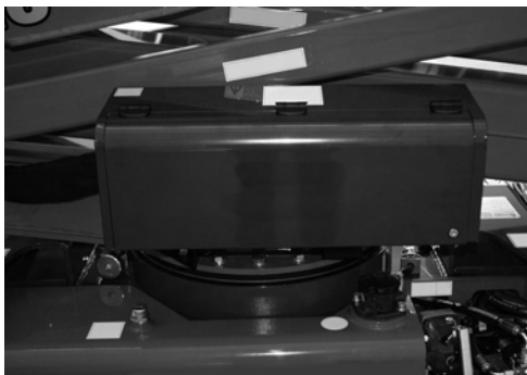
Fig. 109 Aerial part distributor protection
