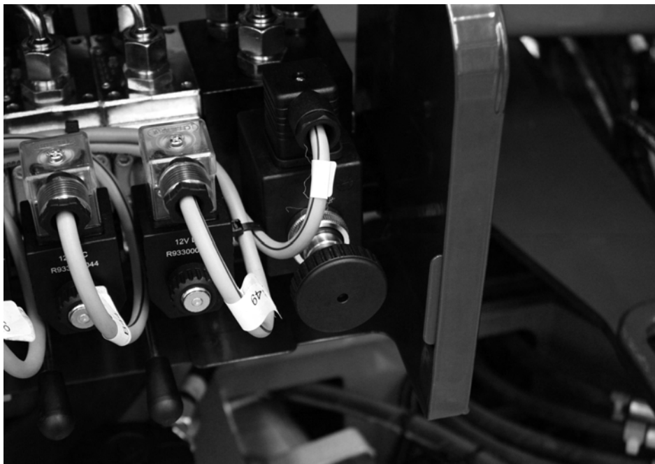
Fig. 75 Knob activation proportional valve aerial part
