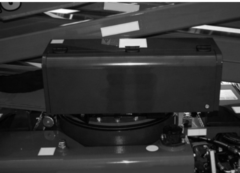
Fig. 121 Aerial part distributor protection
