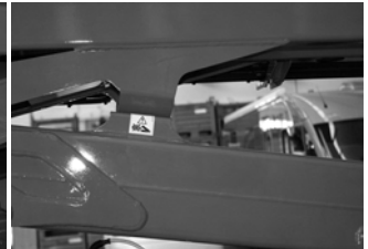
Fig. 97 Example potential shearing risk zone 3
